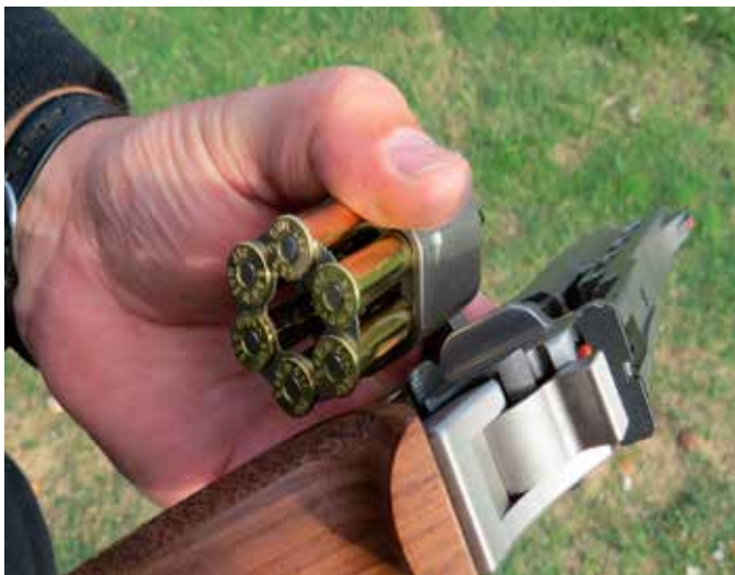
View of moonclip being inserted into the cylinder
