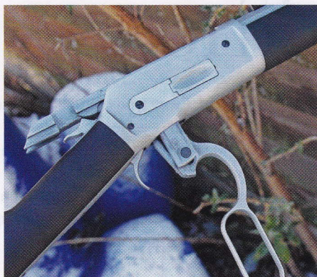
The action shows a solid base for strength, you need to hit that lever hard to ensure the shell lifter actuated fully
