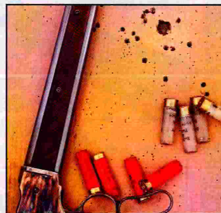
Pounding 00 buckshot loads downrange from 45 feet and 15 feet, the sawed off Chiappa 1887 delivered tight groupings with the best measuring 3.25 inches.
