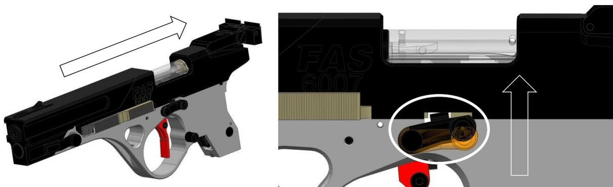
2. When the bolt is in the back position, you can remove the magazine pushing the magazine's button. The magazine is rejected automatically.
