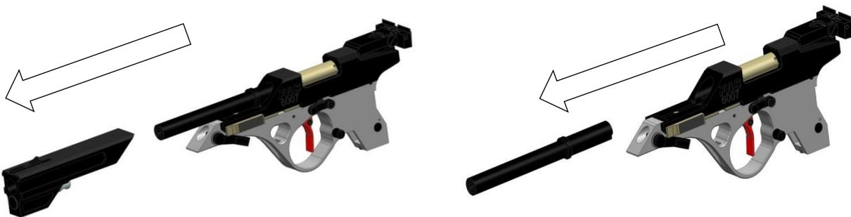
3. pull the rear slide at the front of gun and take out and then take out the bolt
