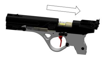
b. Before the round arrives to the ejector, push down ammunition in order to unhook the ammunition from the extractor
