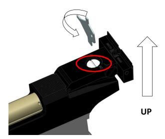
3. To open the width of rear sight, screw the "width screw"; to close the width of rear sight, unscrew the "width screw".
