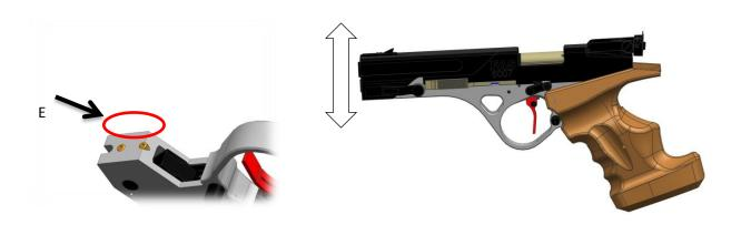
3. Turn counterclockwise the screw (F) to turn right the pistol, or turn counterclockwise to turn left the pistol
