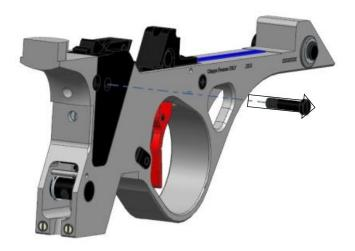
2. Take out from the top of gun the hammer group container's. Pay attention to the transmission lever, it is engaged into hammer group container's.
