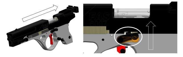
2. When the bolt is in the back position, you can remove the magazine pushing the magazine's button. The magazine is rejected automatically.
