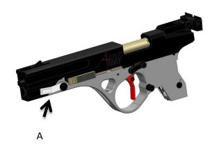
1. With the pistol unloaded, the magazine removed and the hammer down, rotate the lever (A) counterclockwise in order to unlock the slides.
