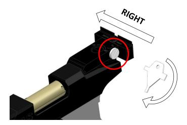
2. To adjust your impact's point to the "up", unscrew the "elevation sight screw"; to adjust your impact's point to the "down", "screw the elevation sight".
