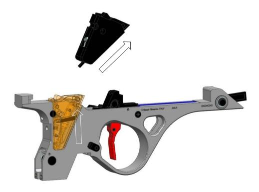
3. Push out the pin and unscrew the screw of trigger group
