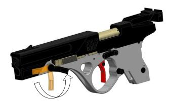
2. Remove the front slide and the barrel
